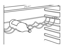
To do this pull the bottle rack forward until it can be tilted upwards, then slide the front support into the next level up.
